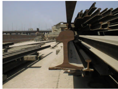
Figure 1: Worn rails replaced from Line No. 2 and stored in Shoubra workshop.
